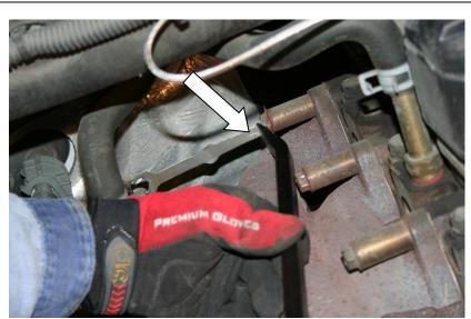
12. Remove the manifold heat shield with a 15mm socket.
