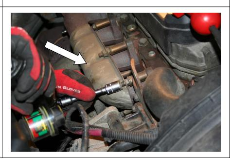
13. Remove the remaining manifold bolts using a 13mm socket.
