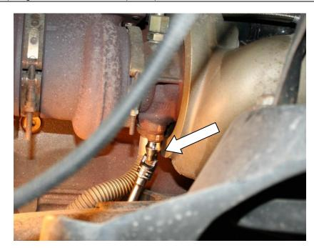
7. Cut the heater pipe bracket to assist in releasing the manifold.
