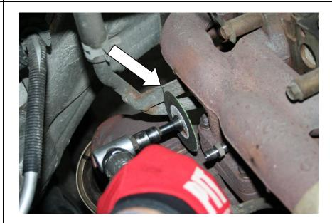
8. Remove turbo oil feed from the turbo.
